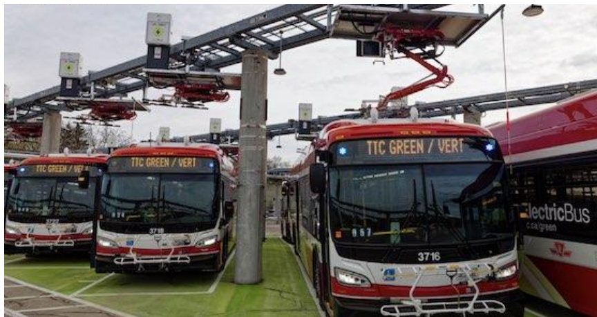
Figure 3. Electric buses at a Toronto Transit Commission (TTC) charging station, equipped with overhead pantograph chargers. 15
